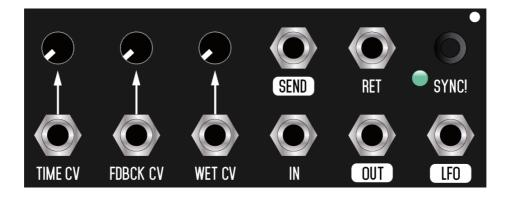
**TIME CV** in: input any signal here to modulate the delay time with something else than the LFO. Try different types of waves, envelopes, S/H outputs, etc. The possibilities are endless. The signal is mixed with the LFO modulation if activated. The small pot sets the amount of modulation.
