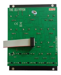
The Jellyfish is designed for Eurorack synthesizer systems and it takes 18HP of space. It requires a -12V / +12V vlagus (2×5 connector), consuming 60mA from the +12V rail and 30mA from the -12V rail. The red stripe of the ribbon cable must be oriented on the same side as the "RED HERE" marking on the printed circuit board.
